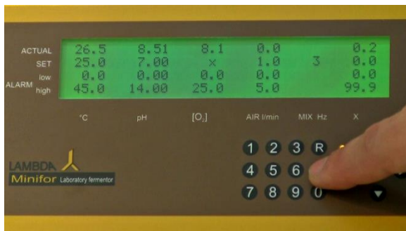
Figure 4 Press button “C” on the MINIFOR control panel to enter the Calibration mode to set or control the address of the MINIFOR for PC control
