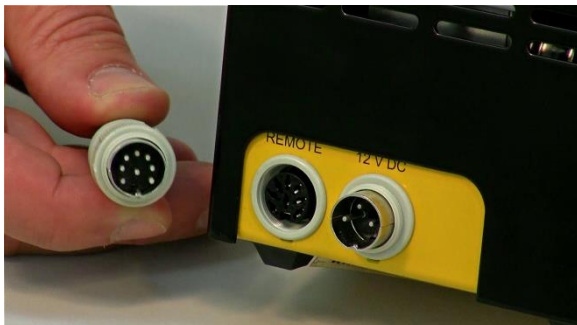
Figure 6 Disconnect the 8-pole remote control cable from the peristaltic pump. While keeping the direction button ◀▶ pressed connect the 8-pole cable to pump again
