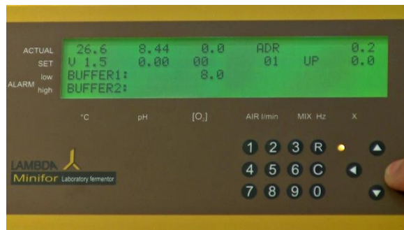
Figure 5 ADR on the Air l/min parameter is the address of the MINIFOR fermentor-bioreactor unit
