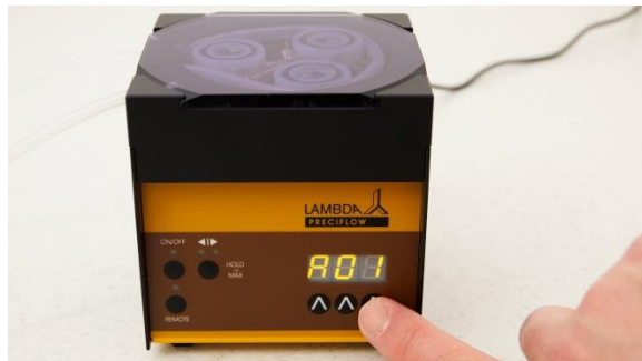
Figure 7 The message “A” and two numbers will appear on the display which correspond to the current address of the pump. Press the buttons ▲▲▲ under the display to modify the address. Press the ON/OFF button to save the set address.
