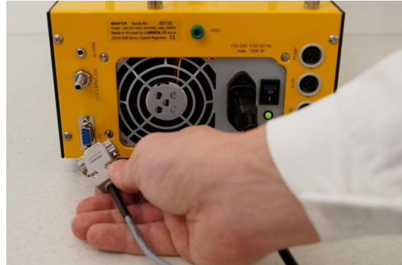
Figure 2 Connect the PC connection cable to the DB 9 connector at the rear of the MINIFOR control unit.
